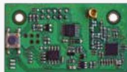
**Internal wireless access point** allows you to connect up to 16 RadioNodes to the main station.
