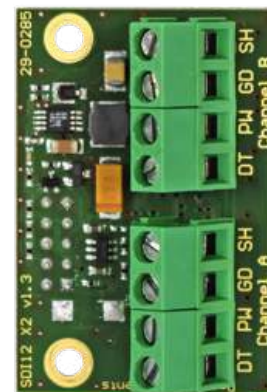
SDI12_X2 Internal Interface for 2 Soil Moisture Probes
